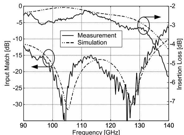
Fig. 10: Simulated and measured microstrip meander line performance
