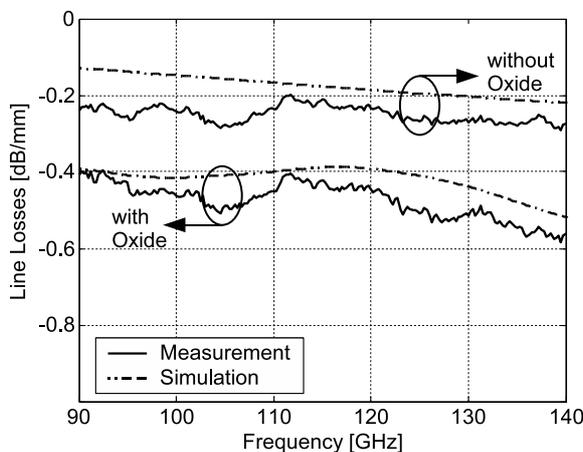
Fig. 8: Losses for a simple microstrip transmission line
