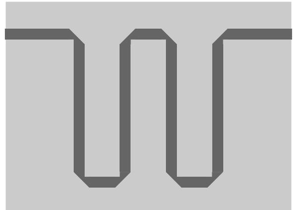
Fig. 9: Layout of a microstrip meander line
