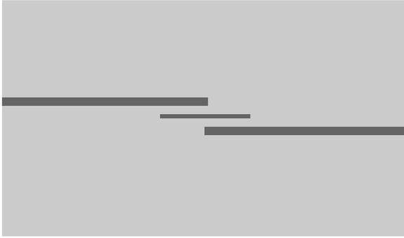
Fig. 11: Layout of the single-pole microstrip filter
